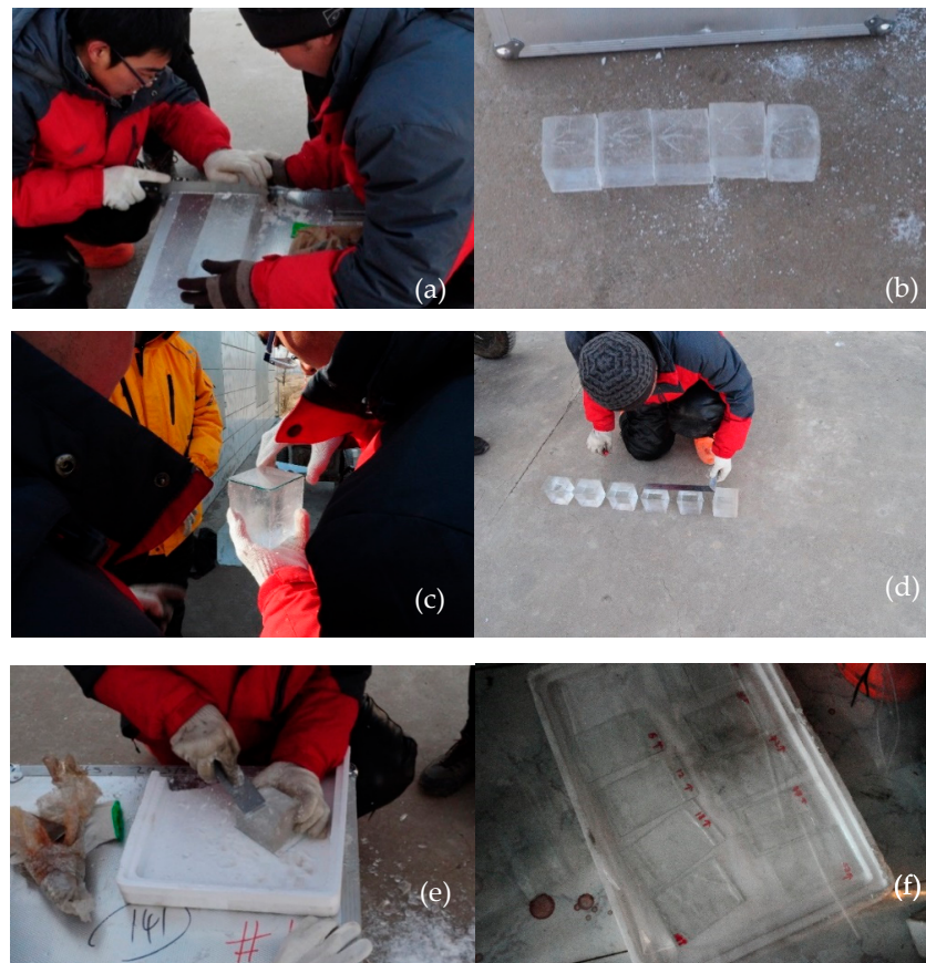
Figure 2. Preparation process of ice slices: (a) sawing ice; (b) labeling ice samples; (c) adhering ice samples to glass sheets; (d) checking adhesion of ice blocks; (e) planning an ice slice; (f) well-polished ice slices.
