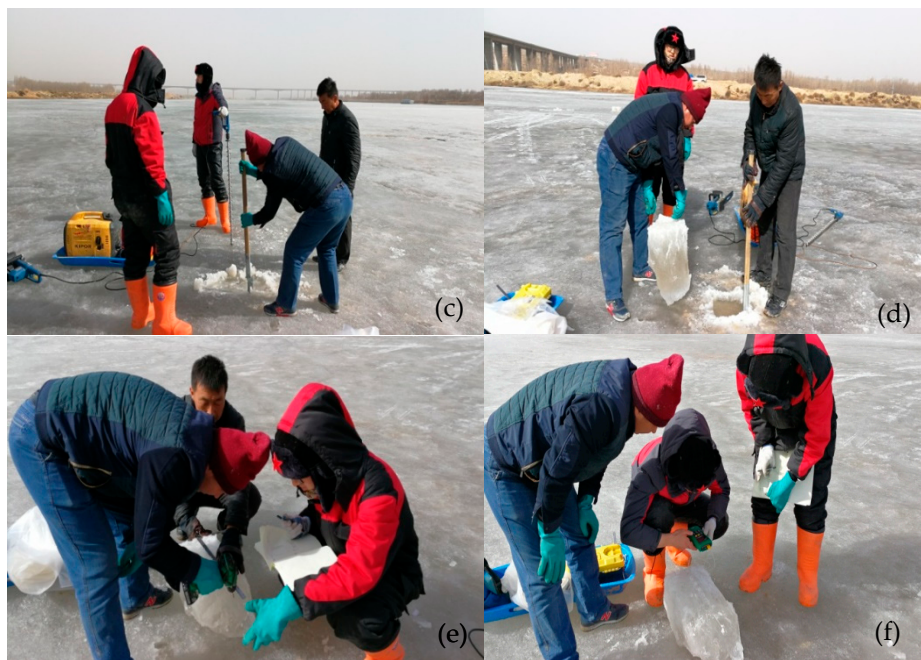
Figure 1. The whole process of ice sample collection: (a) cutting with an electric saw; (b) drilling ice; (c) cutting with a plate saw; (d) ice sample; (e) ice thickness measurement; (f) temperature measurement in ice.
