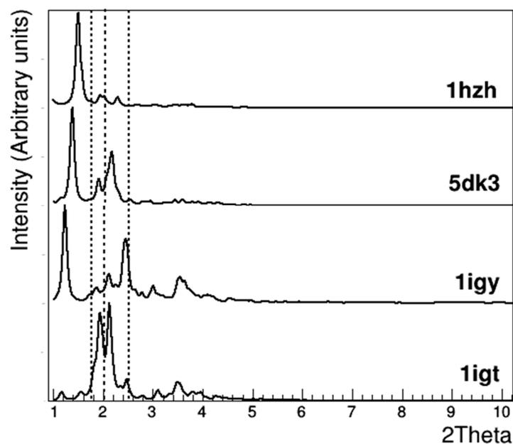
**Figure 3.** Powder diffraction profiles calculated at the same wavelength (2.06642 Å) from the crystal structures of whole monoclonal antibodies (mAb) currently present in the Protein Data Bank, listed in Table 1, which were ordered according to the crystal cell volume, going from bottom (smaller volume) to top (larger volume). Dashed lines indicate the  $2\theta$  values of the diffraction peaks found in powder diffraction profiles from anti-CD20 crystals.
