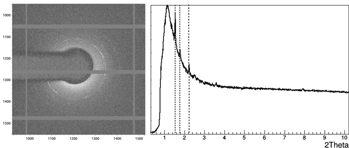
**Figure 2.** Anti-CD20 diffraction image. Noisy and dead detector pixels were masked by choosing proper threshold cut-offs (left), and image intensities were azimuthally integrated to produce a one-dimensional powder diffraction pattern (right).
