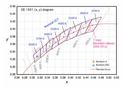
**Figure 4.** The chromaticity tolerance with quadrangle range for LED products in the CIE 1931 chromaticity diagram.
