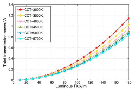
**Figure 6.** Total transmission power comparison for the proposed optimal power allocation strategy under different CCT values with interference coefficient  $\tau = 0.05$ .
