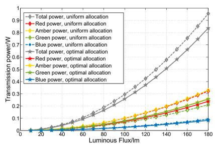
Figure 5. Transmission power comparison between the proposed optimal power allocation strategy and the uniform power allocation method with interference coefficient  $\tau = 0.05$  under CCT = 5700 K.
