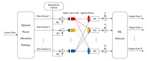
**Figure 1.** CMIMO model for the multi-color light-emitting diodes (LED) based visible light communication (VLC) system.
