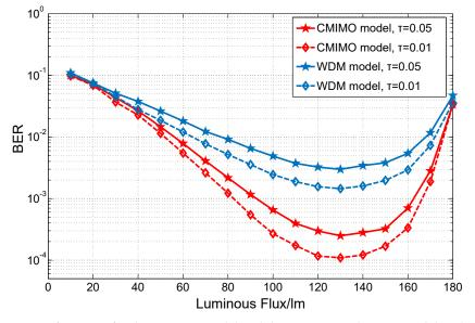
**Figure 7.** Error performance for the CMIMO model and the conventional WDM model under different interference coefficient under CCT = 5700 K.
