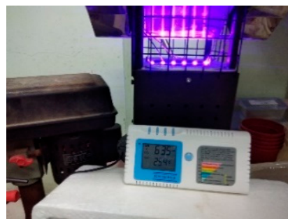
Figure 13. Detection and recording of \text{CO}_2 concentration.
