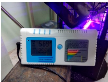
Figure 13. Detection and recording of \text{CO}_2 concentration.
