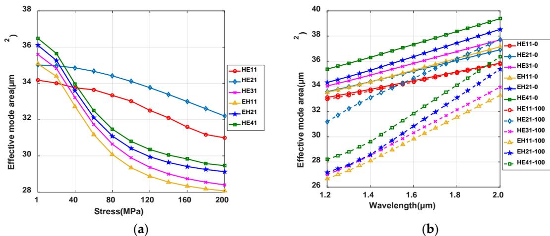
**Figure 15.** (a) Effective mode area as a function of stress for different modes, and (b) effective mode area as a function of wavelength for different modes under 100 MPa stress in the  $y$  direction.
