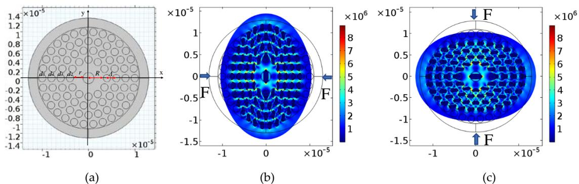
**Figure 2.** (a) Hollow-core C-PCF cross section without stress; (b) hollow-core C-PCF deformed under  $x$  direction external force; (c) hollow-core C-PCF deformed under  $y$  direction external force
