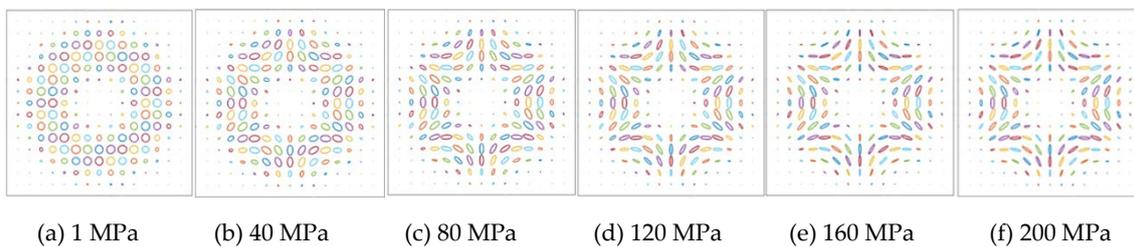
**Figure 12.** Polarization distribution of HE31 mode under stress from 1MPa to 200 MPa in the  $y$  direction.
