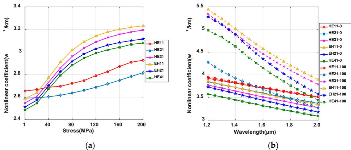
**Figure 16.** (a) Nonlinear parameter as a function of stress for different modes, and (b) nonlinear parameter as a function of wavelength for different modes under 100 MPa stress in the  $y$  direction.
