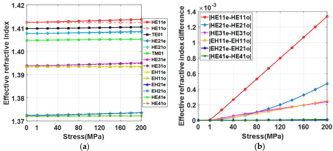
Figure 3. (a) Effective refractive index as a function of stress for different modes; (b) effective index difference between even and odd modes as a function of stress.
