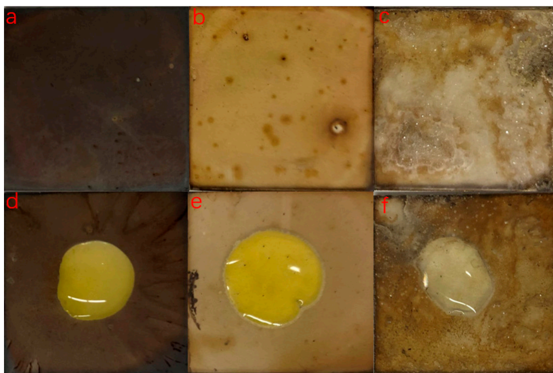
Figure 2. Water-induced degradation experiments ((a–c) are the original images of sample A, B and C before introducing water; (d–f) are the water-contact results of sample A, B, C after 1 s, 10 s, 60 min).
