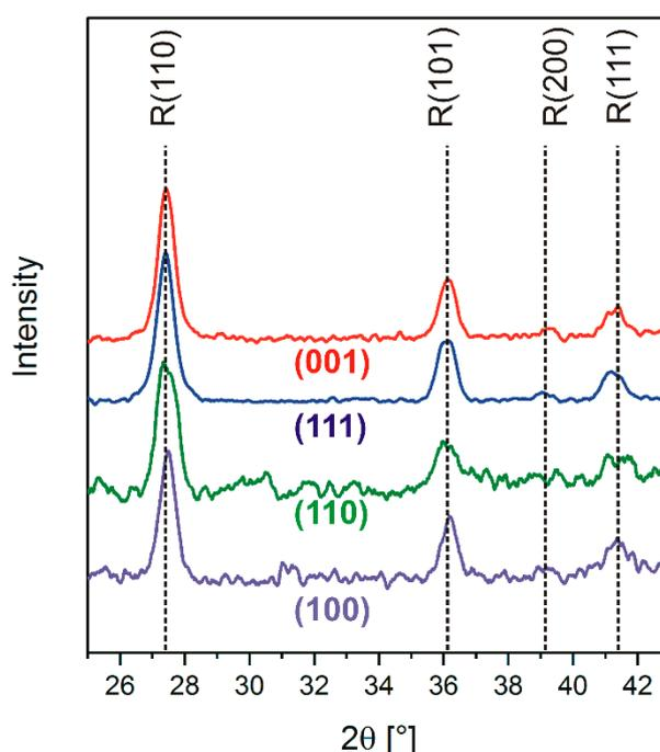
Figure 1: XRD pattern of the hydrothermally grown films on rutile (001), (111), (110), and (100) single crystals. To optimize the surface sensitivity an incident angle of 2° was used during the measurement. The diffraction pattern shows only peaks for rutile TiO<sub>2</sub> labelled with R(110), R(101), R(200), and R(111). Additionally, the existence of any other TiO<sub>2</sub> morphology is excluded. The diffraction patterns are normalized for the R(110) reflex.
