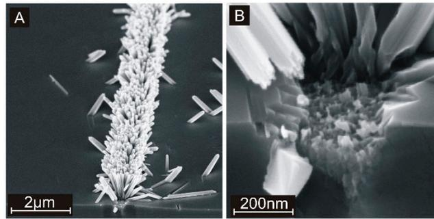
Figure 3: A) SEM cross-section image of an expanded defect on a {110} single-crystalline rutile  $\text{TiO}_2$  substrate. B) Zoom of the cross-section in Panel A.
