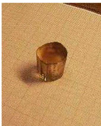
**Figure 21.** TiO<sub>2</sub> grown with no rotation.
