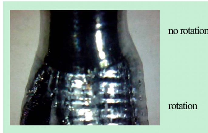
**Figure 22.** Crystal  $\text{Sr}_2\text{Fe}_2\text{O}_5$  grown with no rotation on top of the crystal tube and with rotation on the bottom. (Crystal diameter 8 mm.).
