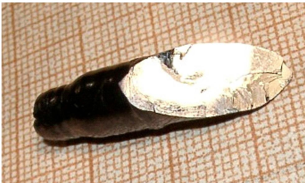
Figure 39. Crystal of  $\text{CoWO}_4$  (growth in air, speed 6 mm/h).
