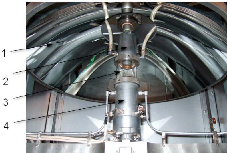
**Figure 13.** High-pressure crystallization chamber. 1. Upper ellipsoidal mirror, 2. Upper flange, 3. Sapphire tube of crystallization chamber, 4. Lower flange.
