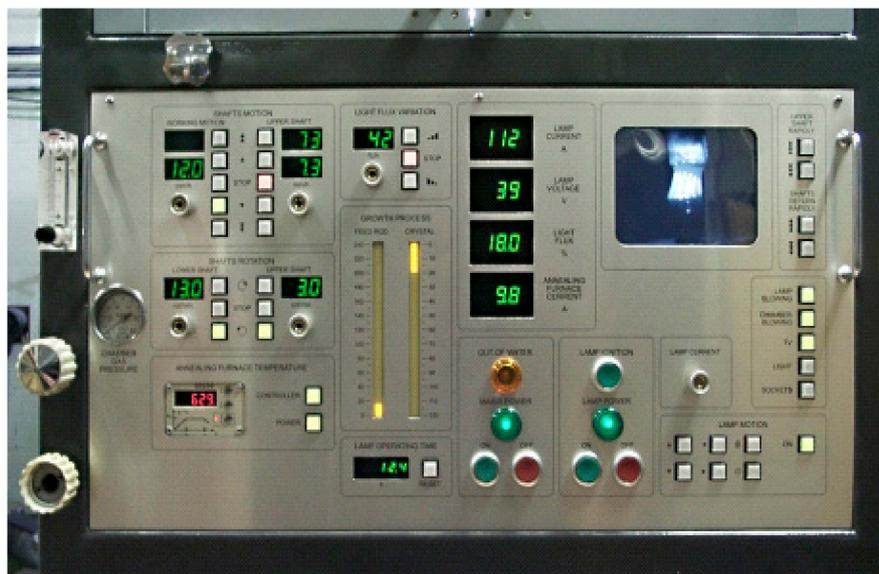
Figure 18. Manual control panel for FZ URN-5-ZM.
