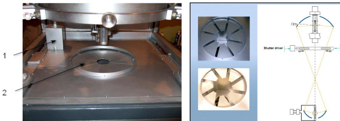
**Figure 19.** The light shutter of FZ URN-5-ZM. 1. Shutter driver, 2. Moving sectors.
