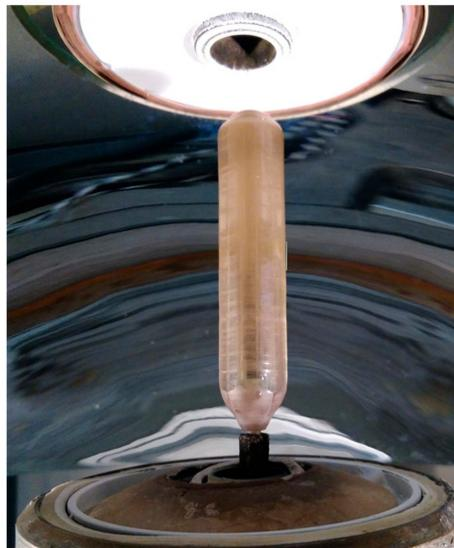
**Figure 28.** Rutile single crystal after crystal growth and annealing immediately. The diameter equals to 20 mm.
