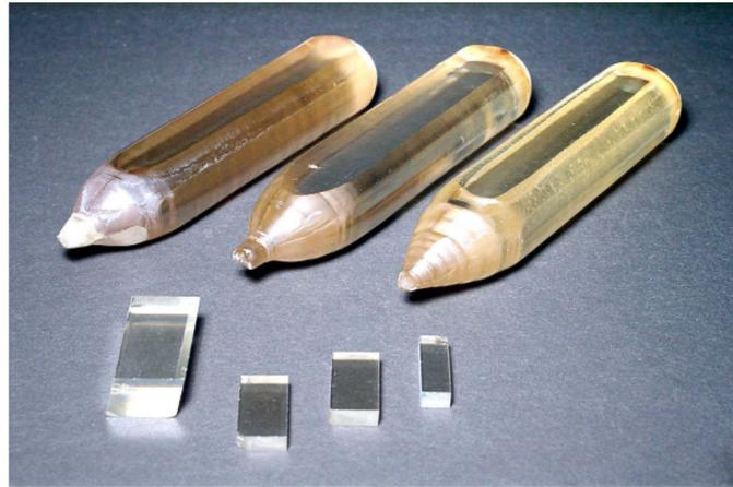
**Figure 27.** Single crystals of rutile are about 20 mm in diameter and small fragments of rutile.
