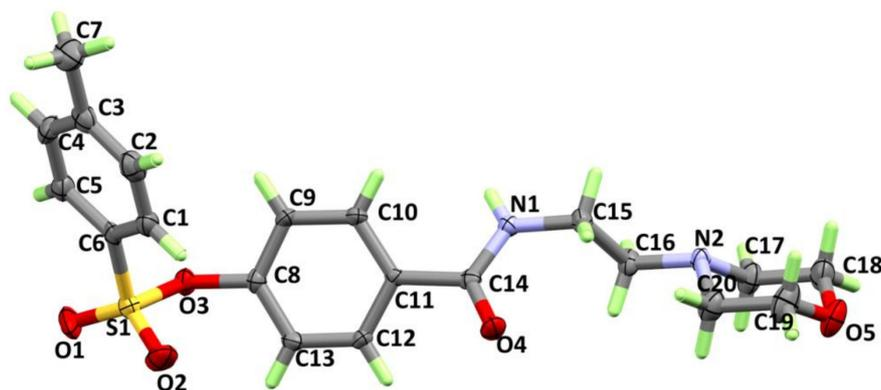
Figure 4. Atom numbering and thermal ellipsoids at a 30% probability level for 7a.
