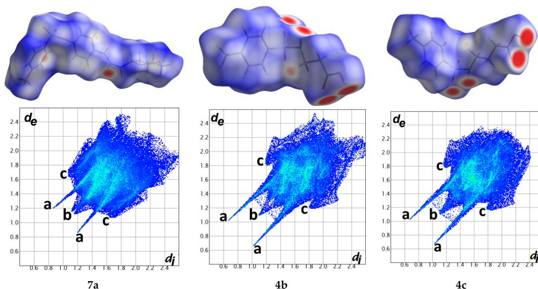
**Figure 5.** The  $d_{\text{norm}}$  surfaces (upper) and fingerprint plots (lower) of the studied compounds. The Sharpe spikes refer to the strong O . . . H hydrogen bonding interactions (a), while the broad peaks refer to the weak hydrophobic C . . . H (b) and H . . . H (c) contacts.
