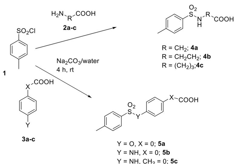
**Scheme 1.** Synthesis of sulfonamide amino acid and sulfonate derivatives.
