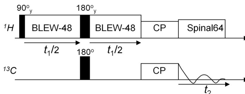
**Figure S2.** PDLF pulse sequence to record dipolar  $^{13}\text{C}$ - $^1\text{H}$  spectra.
