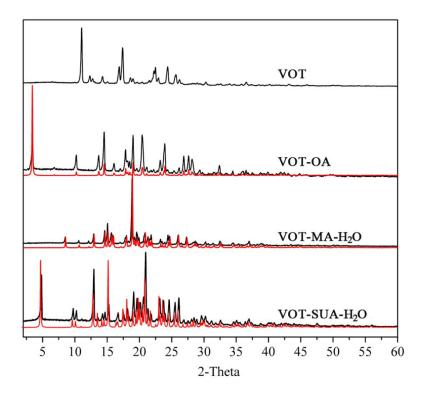
**Figure 6.** Experimental (black) and simulated (red) powder X-ray diffraction patterns for VOT, VOT-OA, VOT-MA-H<sub>2</sub>O, and VOT-SUA-H<sub>2</sub>O salt.
