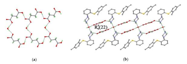
**Figure 4.** (a) Two SUA anions and one water molecules form a sheet-like structure through O5-H5A···O4 and O2-H2···O3 hydrogen bonds; (b) The  $R_6^6(22)$  motif structure are connected by N1<sup>+</sup>-H1A···O1 and N1<sup>+</sup>-H1B···O5 hydrogen bonds.
