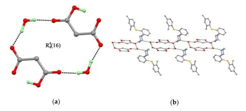
**Figure 3.** (a) Two MA anions and two water molecules form a tetrameric  $R_4^4(16)$  motif through O5-H5A…O1 and O5-H5B…O2 hydrogen bonds; (b) The two-dimensional structure is connected by N1<sup>+</sup>-H1A…O5 and N1<sup>+</sup>-H1B…O2 hydrogen bonds.
