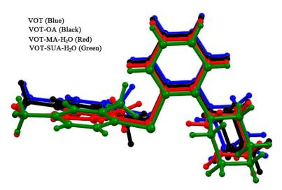
**Figure 5.** Overlay of VOT molecules extracted from crystal structures. Color codes: blue = VOT; black = VOT-OA (1:1); red = VOT-MA-H<sub>2</sub>O (1:1:1); green = VOT-SUA-H<sub>2</sub>O (1:1:0.5).
