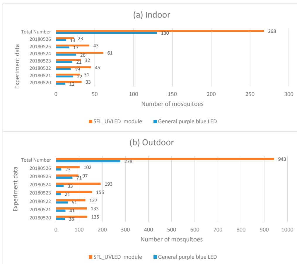
Figure 10. Comparison of (a) indoor and (b) outdoor test results of purple blue LED mosquito trapper and UV LED mosquito trapper with 150° SFL module.
