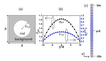
**Figure 1.** (**a**) The unit cell consists of rod and background; (**b**) Curves of effective refractive index and dielectric rod radius varying with Y direction (**c**) Schematic diagram of single layer structure.
