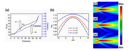
**Figure 5.** (a) The FL and FWHM changes with rotation angles; (b) Effective refractive index profile of GPC lens for LC with different rotation angles. The electric field intensities distributions of micro-lens with rotation angle at (c)  $\theta = 10^{\circ}$  (d)  $\theta = 20^{\circ}$  (e)  $\theta = 30^{\circ}$ .
