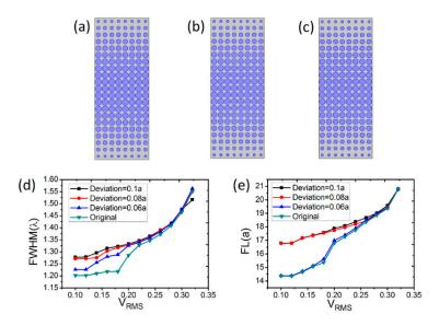
**Figure 7.** Schematic diagram of a cylindrical radii deviation of (**a**) -6% (**b**) -8% (**c**) -10%. (**d**) The FWHM and (**e**) the FL curves with the RMS voltage variation under different deviations.
