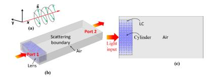
**Figure 3.** (**a**) The direction of the magnetic field vibration in the light wave. (**b**) 3D structure model (**c**) 2D structure model.
