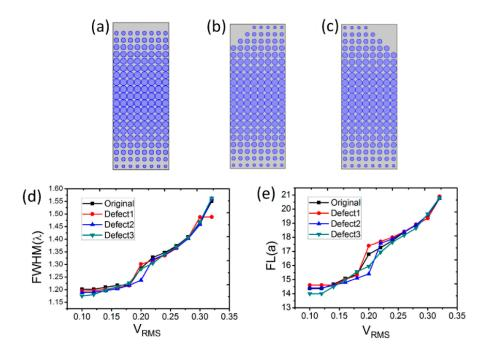
**Figure 6.** Schematic diagram of defects for (**a**) lack of a row of rod on the edge (**b**) lacking of a corner at the front (**c**) lacking of a corner at the back; (**d**) The FWHM and (**e**) the FL curves with the RMS voltage variation under different defects.
