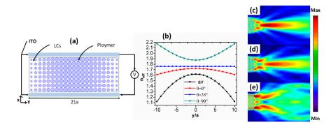
**Figure 4.** (a) The schematic of electrically tunable micro-lens. (b) Effective refractive index distribution with different background of air or LCs with the various of the rotation angles. The electric field intensities of micro-lens with rotation angle of (c)  $\theta = 0^{\circ}$  (d)  $\theta = 38^{\circ}$  (e)  $\theta = 90^{\circ}$ .
