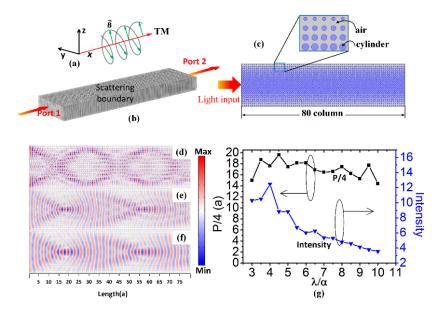
**Figure 2.** (a) The direction of the magnetic field vibration in the light wave (b) 3D structure model of the GPCs (c) 2D structure model of the GPCs. The electric field distributions at (d)  $\lambda/a = 3$  (e)  $\lambda/a = 4$  and (f)  $\lambda/a = 5$  (g). The P/4 and the relative intensity of light at focal point variation with the various of the incident wavelength.
