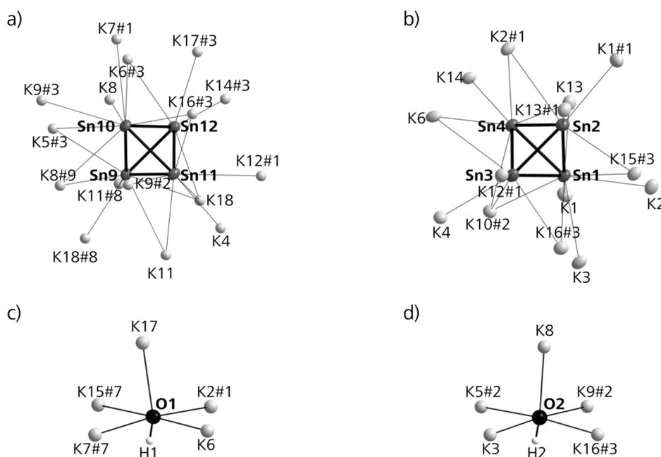
**Figure 7.** Cationic coordination spheres of the two anionic components in  $\text{K}_{4.5}\text{Sn}_4(\text{OH})_{0.5}\cdot 1.75\text{NH}_3$ ; (a)  $[\text{Sn}_4]^{4-}$  surrounded by 16 cations; (b)  $[\text{Sn}_4]^{4-}$  coordinated by 14 cations, as a representative for the other two crystallographically independent  $[\text{Sn}_4]^{4-}$  cages in the asymmetric unit; (c,d) cationic environment of the two hydroxide anions; probability factor: 50%.
