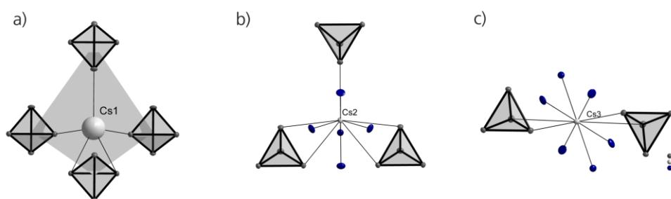
**Figure 2.** Comparison of the cationic coordination spheres of  $[\text{E}_4]^{4-}$  ( $\text{E} = \text{Sn}, \text{Pb}$ ) clusters in  $\text{Na}_4\text{Sn}_4 \cdot 11.5\text{NH}_3$  (a);  $\text{Rb}_4\text{Sn}_4 \cdot 2\text{NH}_3$  (b);  $\text{NaPb}$  (c);  $\text{Rb}_4\text{Pb}_4 \cdot 2\text{NH}_3$  (d) and  $\text{Cs}_4\text{Pb}_4 \cdot 5\text{NH}_3$  (e); probability factor: 50%; dark grey marked cations occupy special *Wyckoff* positions.
