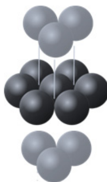
Figure 4. Formation of a hexagonal closest packed (HCP) crystal.
