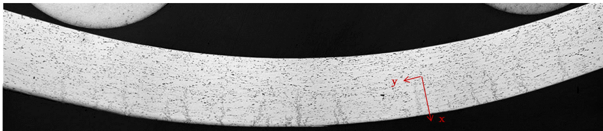
Figure 2. Bright-field optical micrograph of the sample in 4-point bending. The axis in red indicates the orientation of the EBSD measurement.
