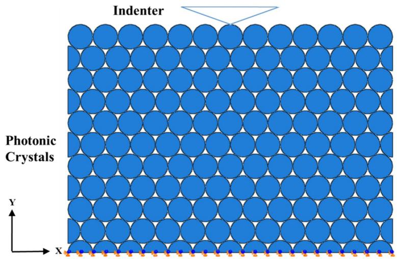
Figure S1. The geometric model of colloidal crystals.
