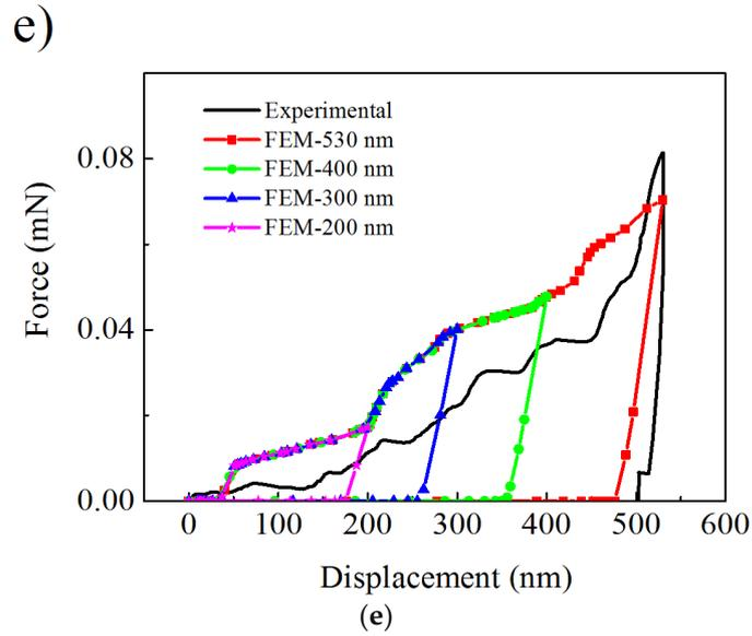
**Figure S2.** The simulation curves under different indentation depth (a) 326nm, (b) 347nm, (c) 438nm, (d) 470nm, (e) 538nm.
