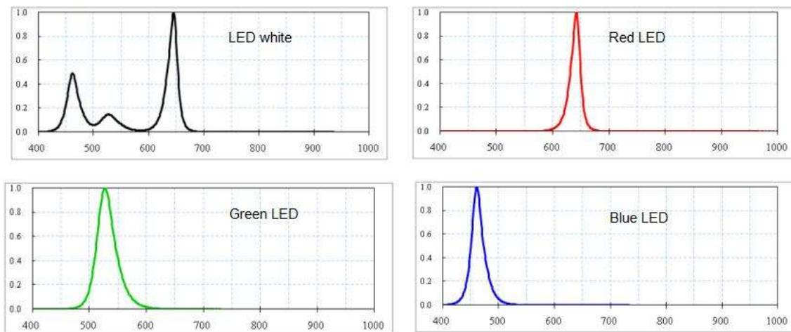
Figure 4. Spectrum distribution of LED light source.
