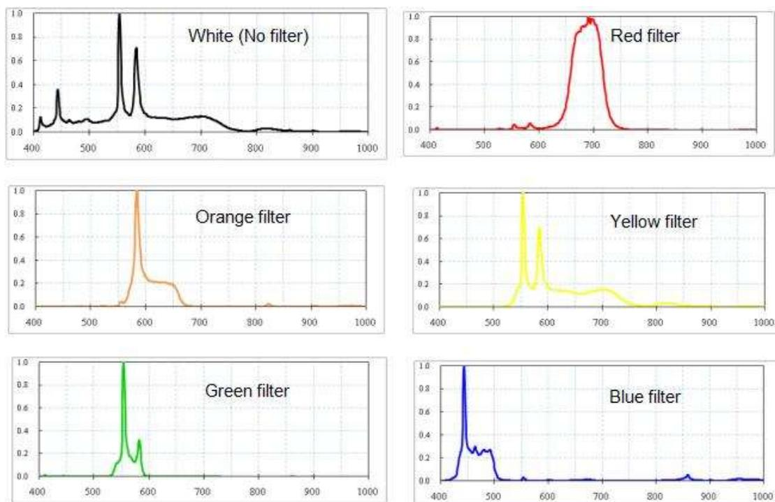
Figure 2. Spectrum distribution of metal-halide light source.
