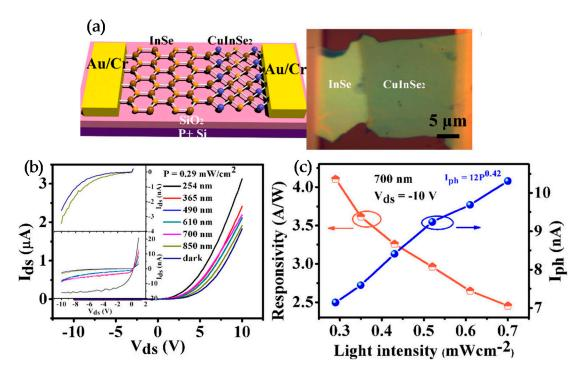
**Figure 5.** (a) Schematic and optical image of a InSe/CuInSe<sub>2</sub> p-n heterostructure. (b) Photocurrent of a p-n diode under various illumination wavelengths at 0.29 mW cm<sup>-2</sup>. (c) Photocurrent and responsivity as a function of optical intensity.
