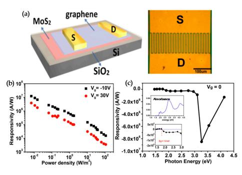
**Figure 2.** (**a**) Schematics of graphene/MoS<sub>2</sub> layered structure. (**b**) photoresponsivity of graphene/MoS<sub>2</sub> photodetectors. (**c**) Light energy-dependent photoresponsivity.
