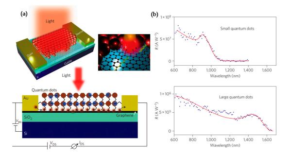
**Figure 1.** (**a**) Schematic of the graphene-quantum dot hybrid phototransistor. (**b**) Spectral responsivity of the hybrid photodetector.
