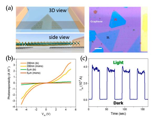
**Figure 6.** (a) Schematic three-dimensional (3D) and optical images of a Gr-WS<sub>2</sub>-Gr photodetector. (b) Photoresponsivity of the four types of detectors. (c) The time-resolved photoresponse of the device.
