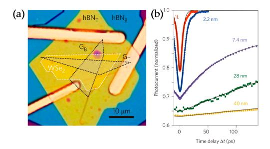
**Figure 7.** (a) Optical image of a heterostructure.  $G_T$  and  $G_B$  are the top and bottom graphene layers, respectively. (b) Time-resolved photocurrent measurements with different layer thicknesses.
