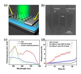
**Figure 9.** Schematic (**a**) and SEM (**b**) image of an Al nanodisk plasmon-enhanced InSe avalanche photodetector. (**c**) Photocurrent spectra of InSe, InSe decorated with Al nanodisks, and Al nanodisk arrays. (**d**) Photocurrent response of the devices.
