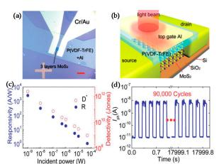
**Figure 8.** Optical (**a**) and 3D schematic (**b**) view of the device. (**c**) Photoresponsivity and detectivity of the device under various incident power. (**d**) Photocurrent response during 90,000 cycles of operation.
