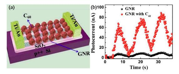
**Figure 4.** (a) Schematic design of the hybrid graphene nanoribbon (GNR)-C60 nanostructure. (b) Time-resolved photocurrent of GNR-C60 hybrid phototransistor and bare GNR phototransistor.
