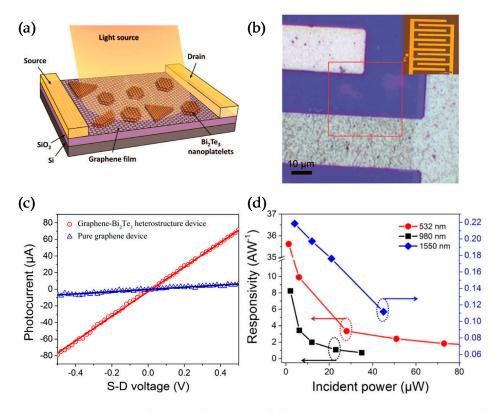
**Figure 3.** Schematic (**a**) and optical (**b**) image of the heterostructure phototransistor device. (**c**) Photocurrent profile with respect to source-drain voltage. (**d**) Device photoresponsivity under different incident power at 532, 980, and 1550 nm, respectively.
