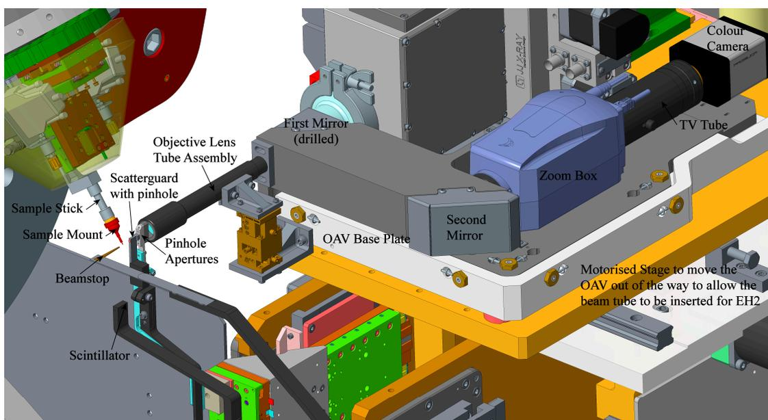
**Figure 6.** Detailed view of the on-axis viewer assembly and beam conditioning “sticks” located in the vicinity of the sample. The  $\omega$ -axis is shown at  $180^\circ$ .
