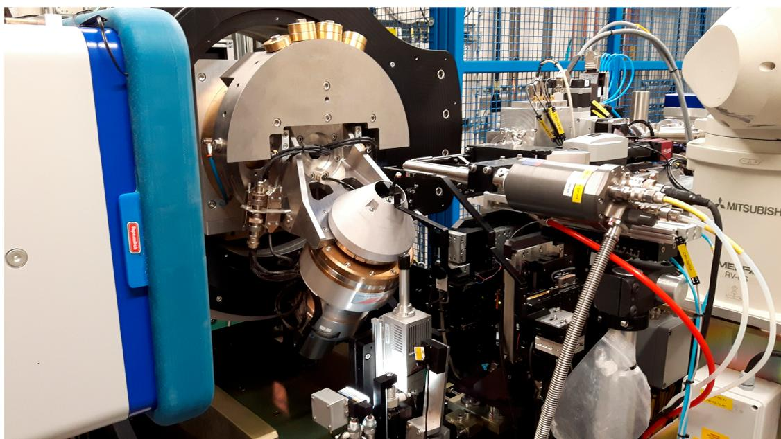
**Figure 9.** The complete diffractometer system in its fully assembled form. The diffractometer is shown with  $2\theta = 0^\circ$ ,  $\omega = 0^\circ$ ,  $\phi = 0^\circ$  and the detector distance set to 300 mm.
