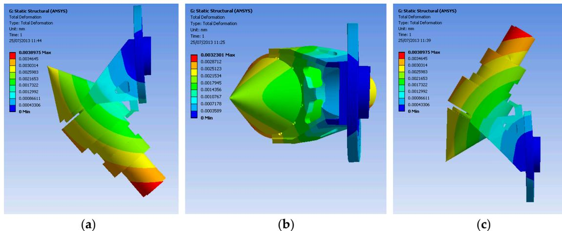
**Figure 4.** Deformation map for the goniometer from the FEA calculations: (a) for  $\omega = 0^\circ$ ; (b) for  $\omega = 90^\circ$ ; and (c) for  $\omega = 180^\circ$ . The scale is shown as the degree of deflection in mm.
