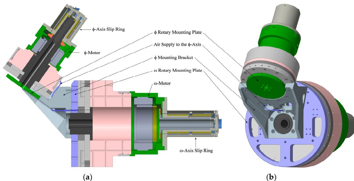
**Figure 3.** The dual air-bearing goniometer. (a) A cut-away view of the air-bearing assemblies showing the paths of the air-flows and cross-sections of both the DC-brushless motors and the electrical slip-rings. (b) A perspective view of the dual air-bearing goniometer detailing the  $\varphi$ -axis bracket.
