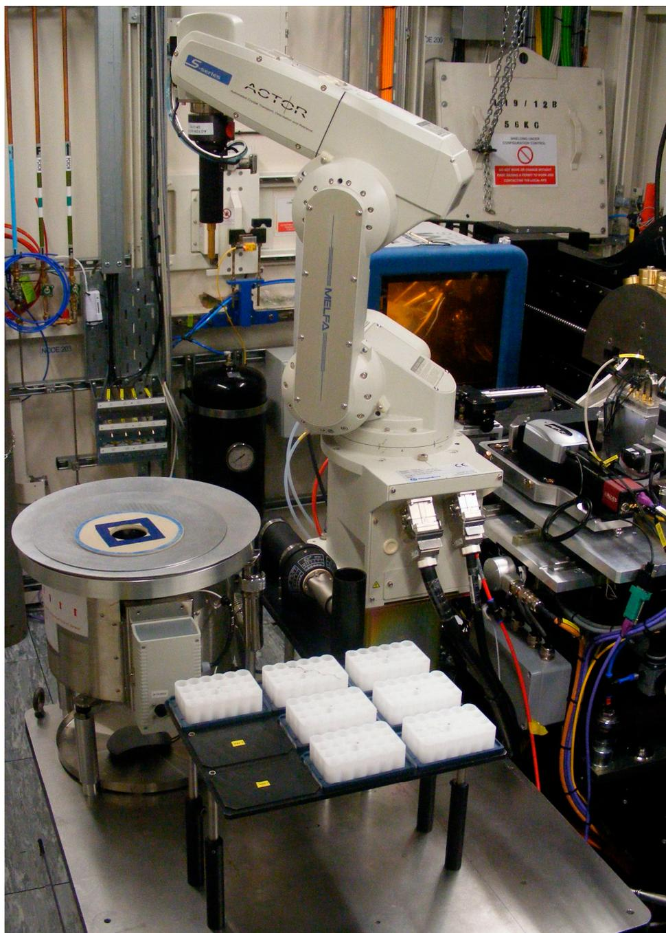
**Figure 8.** The robotic sample changer. The Dewar for storing unipucks is shown to the left of the robotic arm while the trays for holding sample mounts under ambient conditions are shown in the foreground. The aperture in the sliding lid of the Dewar is indicated by a blue square inside a blue circle for the image-recognition system. The camera for locating the lid aperture is mounted above the robot table and not shown here.
