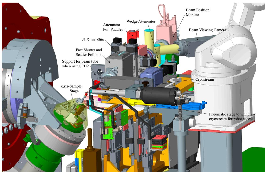
**Figure 5.** Detailed view of the sample stages, on-axis viewer and beam conditioning assembly. The conical cover has been shown as transparent to allow the  $x,y,z$  sample stages to be viewed. The detector has been omitted for clarity.
