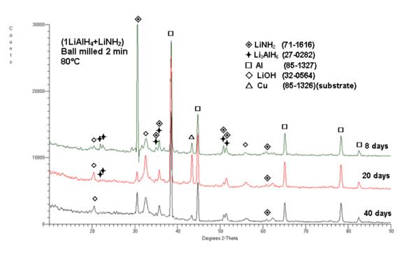
Finally, it must be pointed out that the diffraction peaks of LiOH are also observed in the XRD patterns in Figure 9. LiOH is an impurity, frequently found in LiNH<sub>2</sub> [16]. Alternatively, a part of LiOH might have been formed by oxidation of LiH from reaction (2) in an XRD holder.
