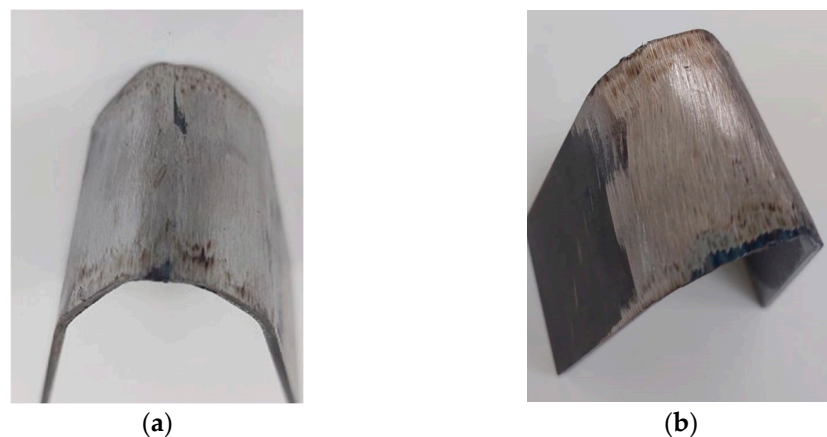
Figure 13. Welded samples of bending test performed with ESAB E6013 electrode (a) and IMAN-9 electrode (b).
