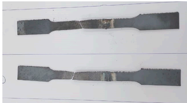
Figure 11. Tensile specimen for welds performed with E 6013 electrode after breaking.
