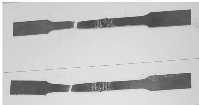
Figure 12. Tensile specimen for welds performed with IMAN-9 electrode after breaking.
