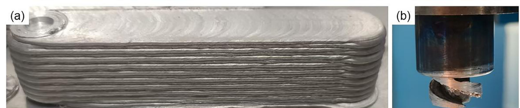
Figure 2. Deposited components: (a) 27-layer deposited component; (b) appearance morphology of the spiral tool after deposition.
