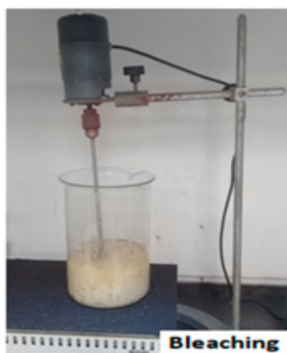
Figure 2. Bleaching treatment under mechanical stirring.
