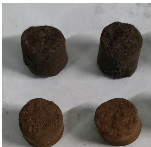
Figure 3. Picture of sintered KSCs at 1150 °C.
