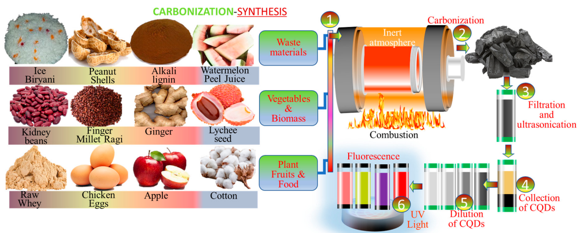
Figure 7. Schematic representation of the synthesis of CDs with the help of the Carbonization synthesis technique.
