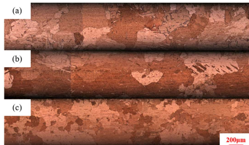
Figure 3. Directional heat treatment microstructure of 89% pure copper wire at 600 °C and different withdrawing velocities: (a) 3 µm/s; (b) 8 µm/s; (c) 20 µm/s.
