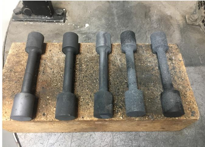
**Figure 3.** One ADI specimen from each set after high-temperature tempering.
