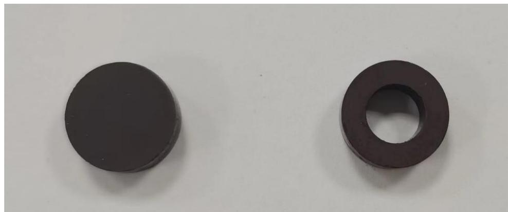
**Figure 8.** Vertical view of the  $0.3\text{H}_3\text{BO}_3\text{-}0.2\text{NaCl-}0.5\text{Ni}_{0.5}\text{Zn}_{0.5}\text{Fe}_2\text{O}_4$  multiphase ceramic sample.
