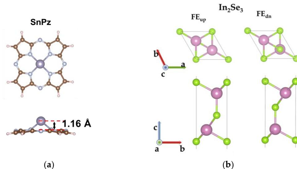
**Figure 1.** (a) The structure of SnPz molecule. (b) The structures of  $\text{In}_2\text{Se}_3$  in case of  $\text{FE}_{\text{up}}$  (left) and  $\text{FE}_{\text{dn}}$  (right).
