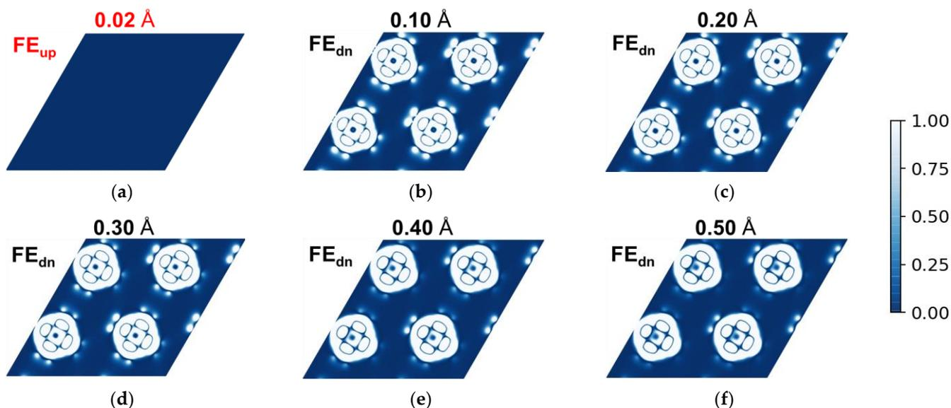
**Figure 6.** (a) STM image of  $SnPz/In_2Se_3$  in the  $FE_{up}$  state, taking the result at the material surface of  $0.2 \text{ \AA}$  as an example. (b–f) STM images of  $SnPz/In_2Se_3$  in the  $FE_{dn}$  state, with probe heights of  $0.1 \text{ \AA}$ ,  $0.2 \text{ \AA}$ ,  $0.3 \text{ \AA}$ ,  $0.4 \text{ \AA}$ , and  $0.5 \text{ \AA}$  from the  $SnPz/In_2Se_3$  surface, respectively.
