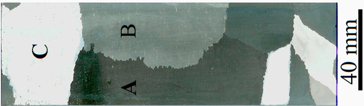
**Figure 10.** The structure and sizes of grains from the DIC assisted CSA method applied to A1050 commercially pure aluminum, for the parameter set ((550 °C, 2 h), 3%, (550 °C, 24 h)).
