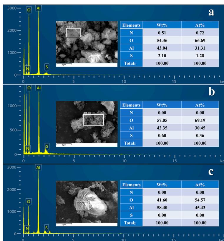
**Figure 6.** The energy spectra of the samples. (a): HT-150-1 h; (b): HT-150-4 h; and (c): HT-150-16 h.
