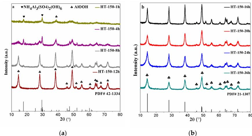
Figure 2. XRD patterns of samples at 150 °C. (a) HT-150-1 h, HT-150-4 h, HT-150-8 h, and HT-150-12 h samples, and (b) HT-150-16 h, HT-150-20 h, HT-150-24 h, and HT-150-36 h samples.
