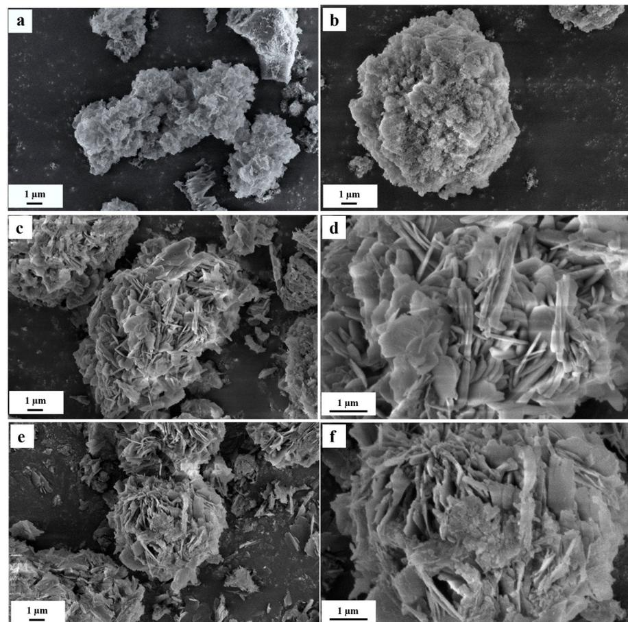
Figure 5. SEM images of the different samples. (a): HT-150-1 h; (b): HT-150-4 h; (c,d): HT-150-8 h; and (e,f): HT-150-20 h.
