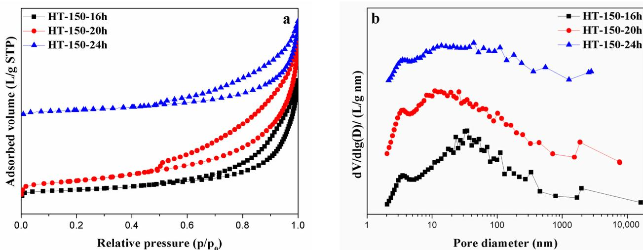
**Figure 7.** N<sub>2</sub> absorption–desorption results of the HT-150-16 h, HT-150-20 h, and HT-150-24 h samples. (a) N<sub>2</sub> adsorption–desorption isotherm; and (b) pore-size distributions.
