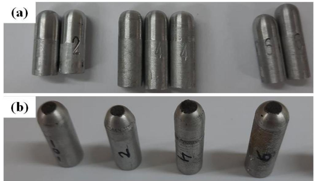
**Figure 4.** Fabricated samples: (a) before wear test; (b) after wear test.
