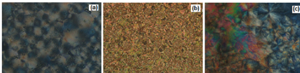
Figure 3. POM textures of 50 mol% of I6/I8 during heating (a) SmB phase at 142 °C; (b) SmC phase at 150 °C; and (c) SmA phase at 158 °C.
