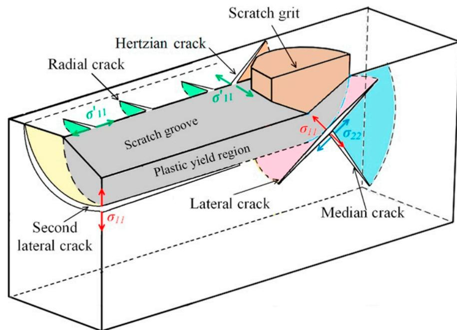
**Figure 4.** Distribution of the stresses and cracks in the single abrasive scratching of fused silica [27].
