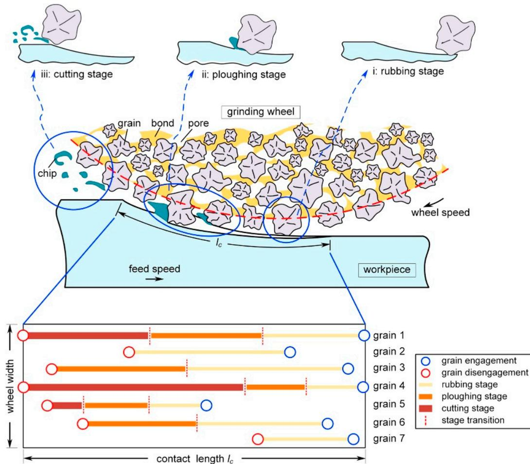
**Figure 2.** Schematics of contact stages between the abrasive grit and workpiece during grinding: rubbing, ploughing, and cutting [5].
