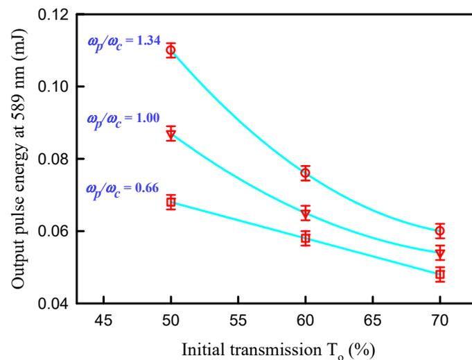
**Figure 3.** Experimental results for the output pulse energy at 589 nm versus the initial transmission  $T_o$  of the saturable absorber for three different pump-to-mode size ratios  $\omega_p/\omega_c$ .
