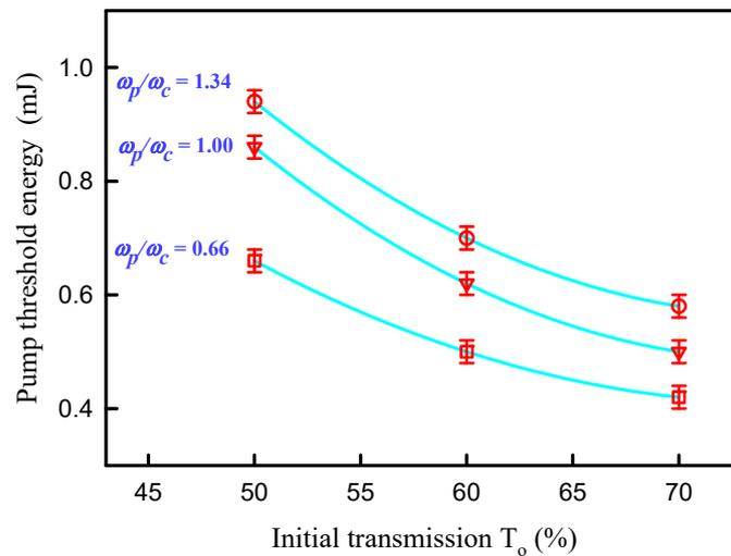
**Figure 2.** Experimental results for the pump threshold energy at 808 nm versus the initial transmission  $T_o$  of the saturable absorber under three different pump-to-mode size ratios  $\omega_p/\omega_c$  for the output pulse rate to reach the pump rate of 10 kHz.
