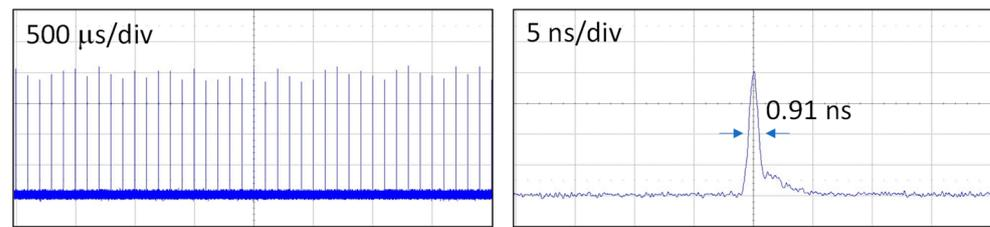
**Figure 6.** Typical pulse train and temporal profile for the orange output at 589 nm obtained with  $\omega_p/\omega_c = 1.34$  and  $T_o = 50\%$ .
