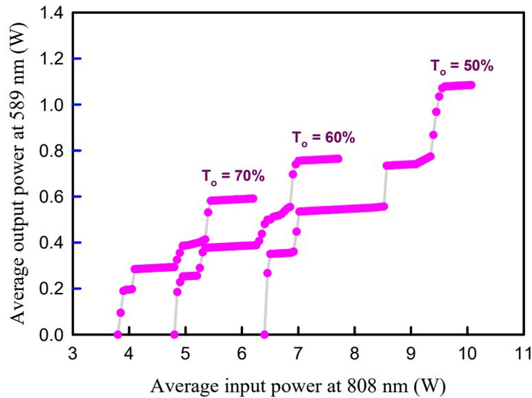
**Figure 4.** Experimental results for the average output power at 589 nm versus the average input power at 808 nm for three different initial transmissions  $T_o$  of the saturable absorbers when  $\omega_p/\omega_c = 1.34$ .
