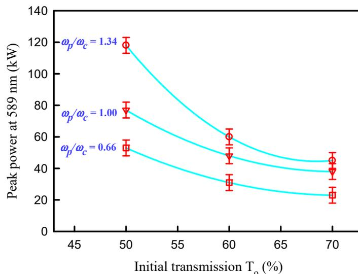
**Figure 7.** Calculated results for the output peak power at 589 nm versus the initial transmission  $T_o$  of the saturable absorber for three different pump-to-mode size ratios  $\omega_p/\omega_c$ .
