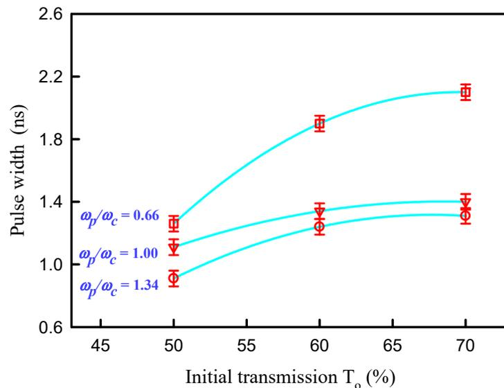
**Figure 5.** Experimental results for the pulse width at 589 nm versus the initial transmission  $T_o$  of the saturable absorber for three different pump-to-mode size ratios  $\omega_p/\omega_c$ .
