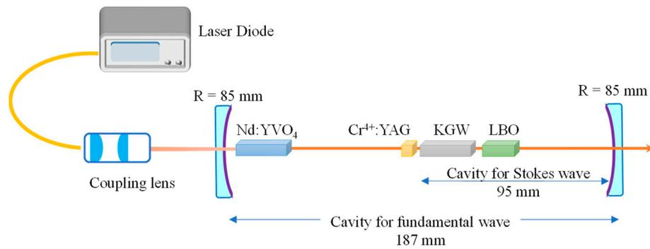
**Figure 1.** Experimental configuration for generating the orange laser at 589 nm in a passively Q-switched Nd:YVO<sub>4</sub>/KGW Raman laser with intracavity SRS and SHG.
