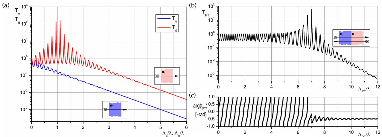
**Figure 4.** Transmittance as a function of ratio  $\Lambda/\lambda$  for: (a) independent gain  $T_g$  and loss  $T_\alpha$  cells; (b) PT cell  $T_{PT}$ . (c) Argument of transmission coefficient  $t_{PT}$  as a function of ratio  $\Lambda_{PT}/\lambda$ .
