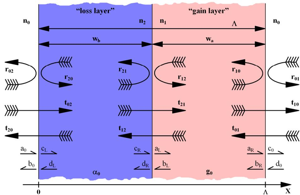
Figure 1. Scheme of the analyzed single primitive cell with PT symmetry.
