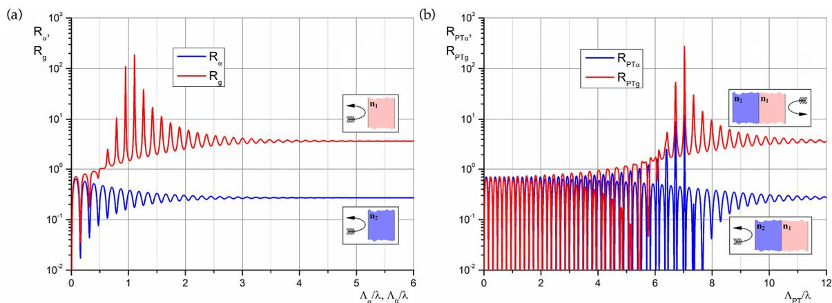
**Figure 3.** Reflectance as a function of ratio  $\Lambda/\lambda$  for: (a) independent gain  $R_g$  and loss  $R_\alpha$  cells; (b) PT gain layer  $R_{PTg}$  and PT loss layer  $R_{PT\alpha}$ .
