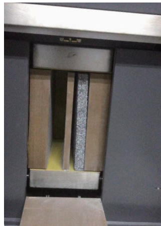
Figure 13. Thermal conductivity test of the GCIB.
