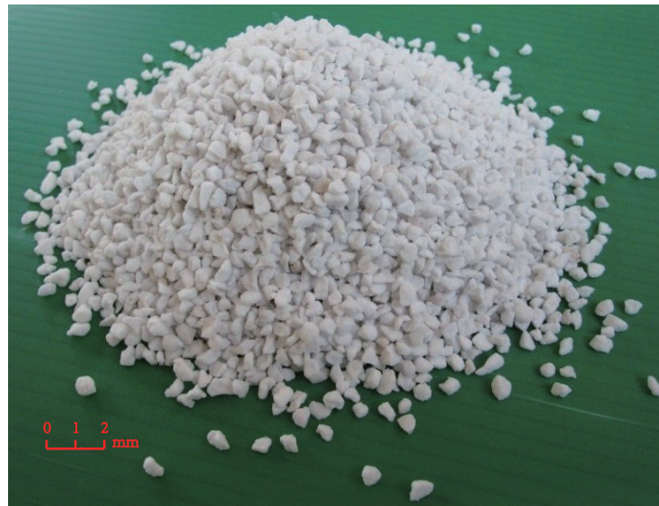
Figure 1. Appearance of vitrified microspheres.
