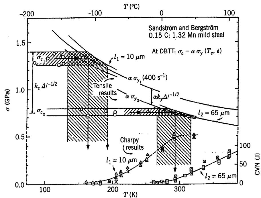
**Figure 4.** A compilation of tensile test and Charpy impact test results obtained by Sandström and Bergström in determining a ductile-to-brittle transition in behavior at two grain sizes [14,15].
