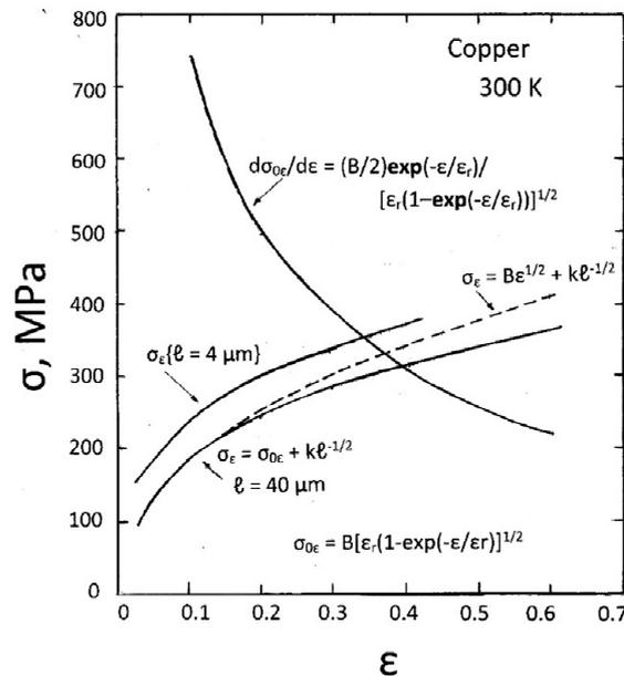
**Figure 2.** H-P based plastic instability computations demonstrating a decrease in the tensile uniform strain at reduced grain size for copper material.
