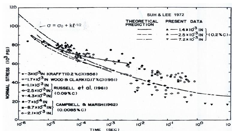
Figure 1. A compilation of delay time measurements for the yielding of carbon steel materials, also with several theoretical model predictions reported by Suh and Lee [9], and also including an extended curve for Hall–Petch dependence;  $10^3 \text{ psi} = 6.9 \text{ MPa}$  and  $1.0 \text{ in} = 2.54 \text{ cm}$ .
