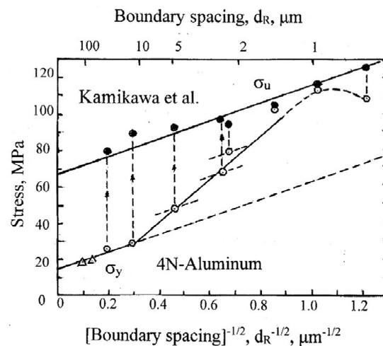
**Figure 3.** The yield stress,  $\sigma_y$ , and true stress at maximum uniform strain,  $\sigma_u$ , for aluminum material as obtained from measurements reported by Kamikawa, Hirooka and Furuhashi [13].
