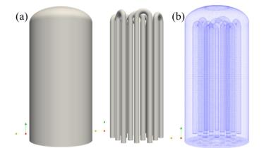
Figure 2. Schematic diagram of furnace body and silicon rods: (a) 3D models; (b) grid structure.
