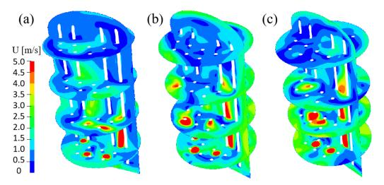
**Figure 6.** Flow field distribution. (**a**) Design A; (**b**) design B; (**c**) design C (height of horizontal sections is the same as in Figure 4).
