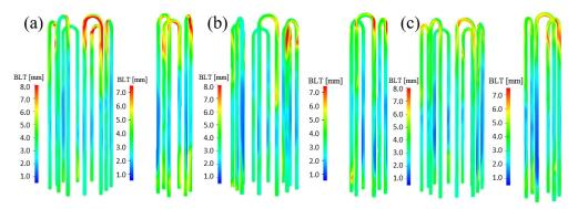
Figure 7. Boundary layer thickness along the rods. (a) Design A; (b) design B; (c) design C.
