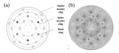
Figure 3. Diagram of base plate: (a) structure; (b) after meshing.
