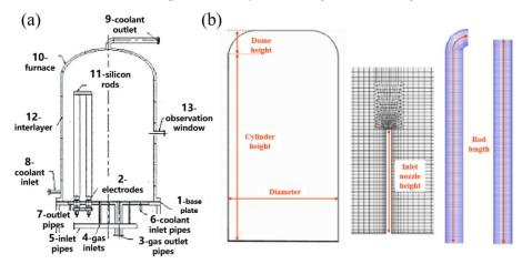
**Figure 1.** Schematic diagram of bell-type polysilicon reduction furnace: (**a**) Profile; (**b**) Furnace shell and silicon rod.
