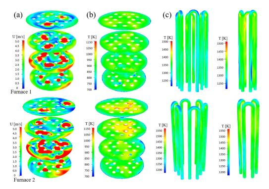
**Figure 9.** Temperature and velocity distributions. (a) Cross-sections of gas velocity; (b) cross-sections of temperature; (c) rod surface temperature (the height of cross-section is 0.5 m, 1.1 m, 1.7 m and 2.3 m, respectively).
