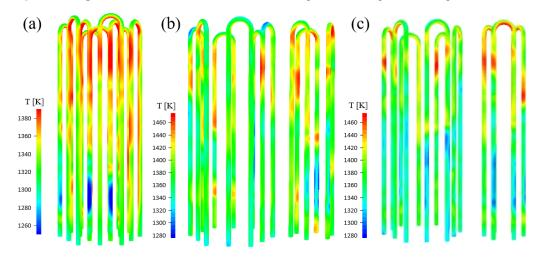
Figure 5. Temperature distribution along rod surface. (a) Design A; (b) design B; (c) design C.
