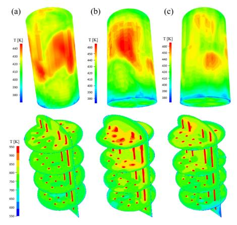
Figure 4. Temperature distribution of furnaces. (a) Design A; (b) design B; (c) design C.
