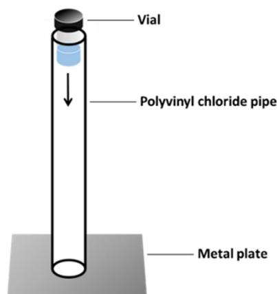
Figure 1. Experimental setup of vial dropping.
