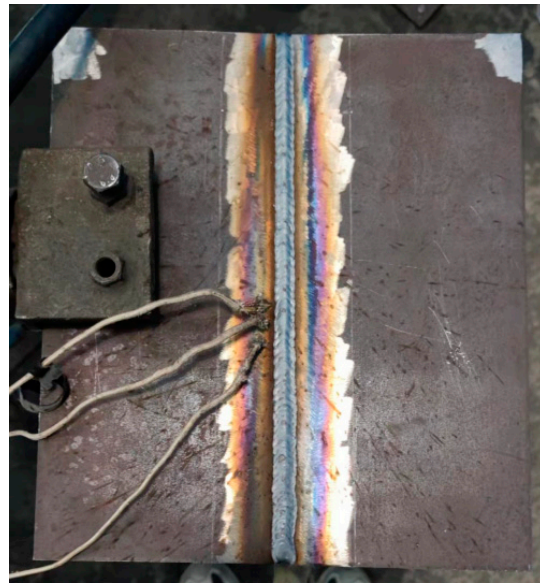
Figure 3. Temperature field measurement.
