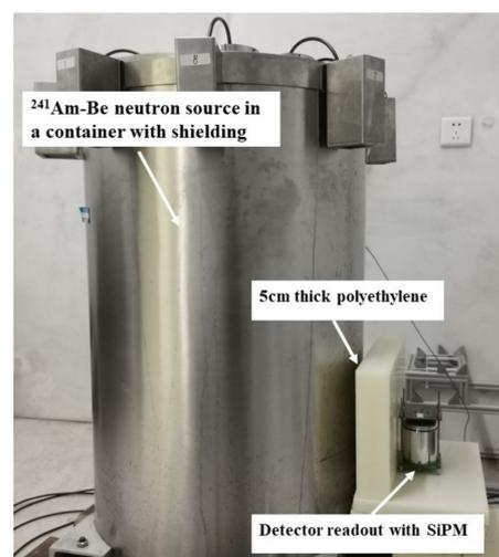
**Figure 3.** Experimental setup with Am-Be neutron source.
