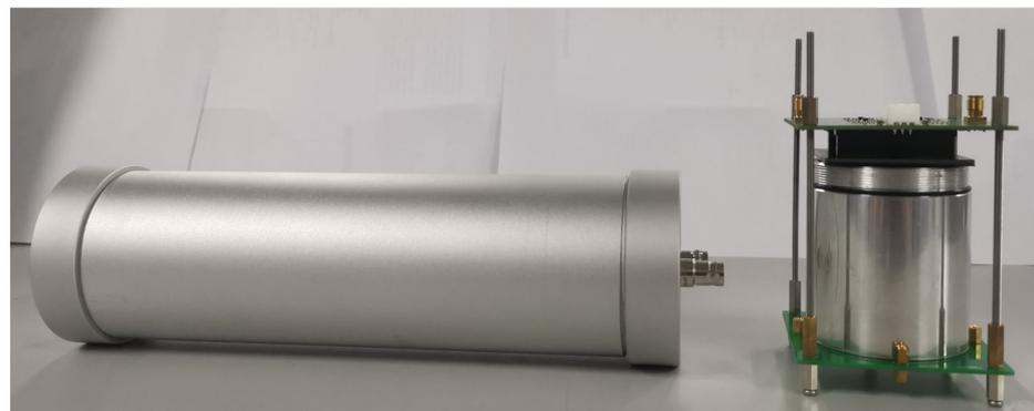
**Figure 1.** Assembly photos of NaIL scintillator readout with PMT (left) and SiPM array (right).
