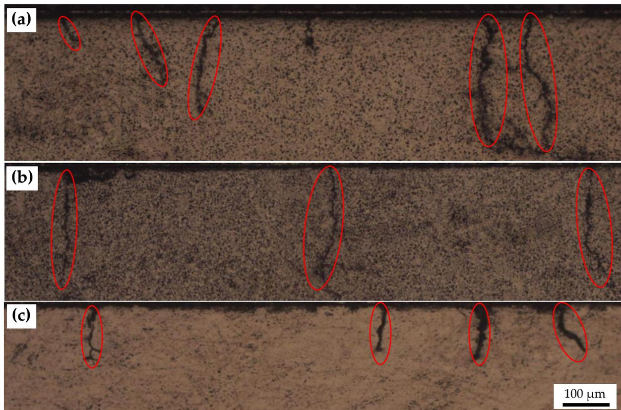
**Figure 7.** Light micrographs of the cross section of WTC samples after thermal loading. (a) As-sintered at 330 MW/m<sup>2</sup>, (b) as-sintered at 440 MW/m<sup>2</sup>, and (c) as-forged at 440 MW/m<sup>2</sup>. The scale indicated is the same for all graphs.
