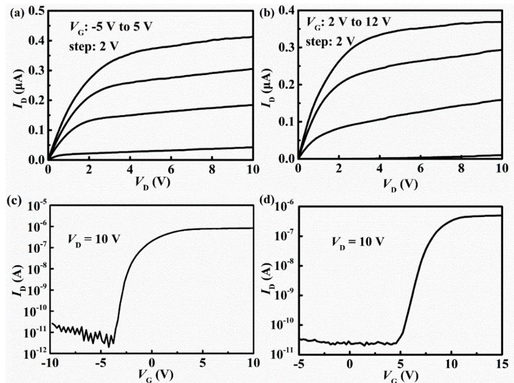
**Figure 5.** (a) Output characteristic curve with various  $V_G$  before and after (b) etching of  $\beta$ -Ga<sub>2</sub>O<sub>3</sub> FET, the transfer curve in log scale before (c) and after (d) etching.
