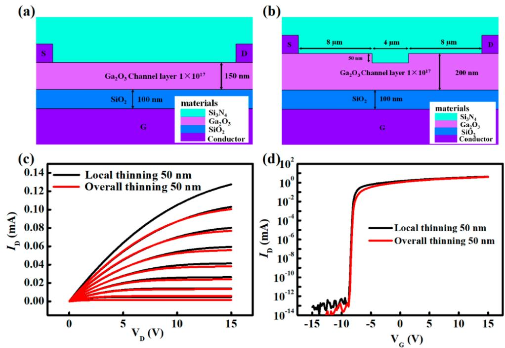
Figure 2. Schematic diagram of the simulation of the overall thinning of 50 nm (a) and the local thinning of 50 nm (b), output characteristic curves (c) and transfer characteristic curves (d) of overall thinning 50 nm and local thinning 50 nm.
