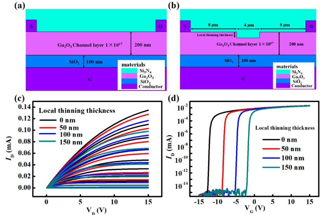
Figure 3. Schematic diagram of the simulation structure of bottom-gate Ga<sub>2</sub>O<sub>3</sub> FET without (a) and with (b) local thinning, output characteristic curves (c) and transfer characteristic curves (d) of different local thinning thickness.
