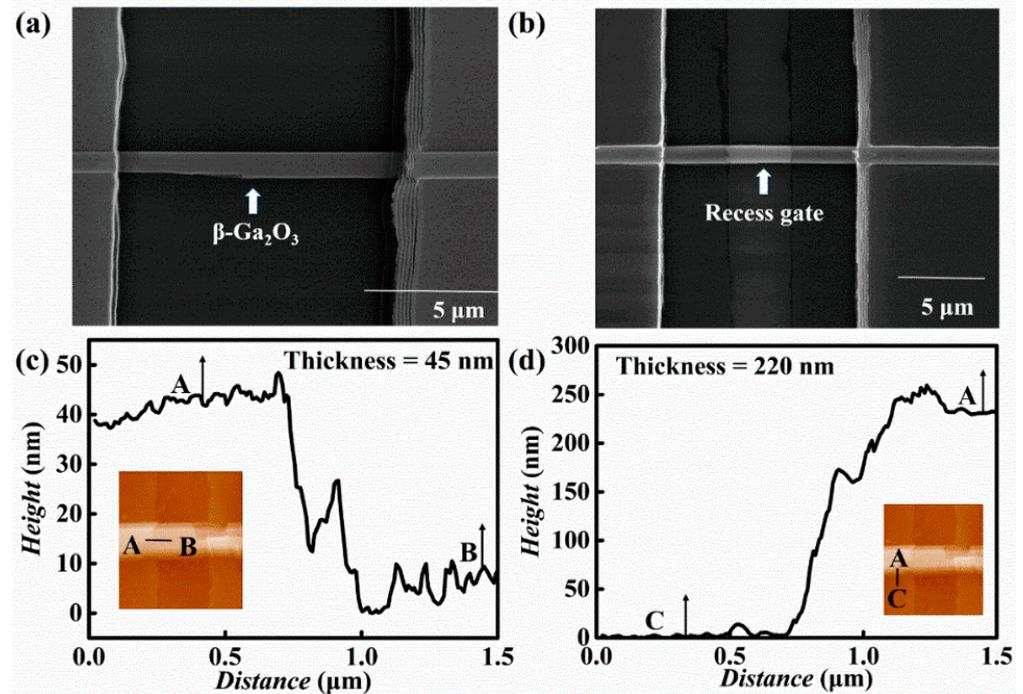
**Figure 4.** (a) SEM image of a  $\beta\text{-Ga}_2\text{O}_3$  thin film made of a FET structure using a Ti/Au electrode, (b) SEM image of the local thinning of a  $\text{Ga}_2\text{O}_3$  FET, (c) AFM height distribution of the local thinning and the  $\text{Ga}_2\text{O}_3$  (d).
