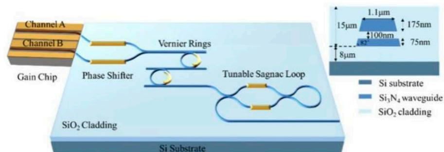
**Figure 12.** Schematic structure of tunable InP–Si<sub>3</sub>N<sub>4</sub> mixed external cavity laser with double parallel gain (the inset shows a cross-section of the Si<sub>3</sub>N<sub>4</sub> waveguide).
