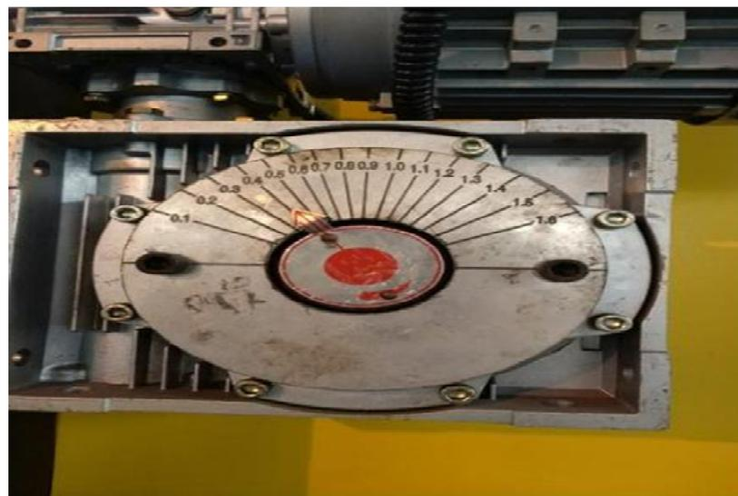
Figure 5. Shear blade clearance setting dial.
