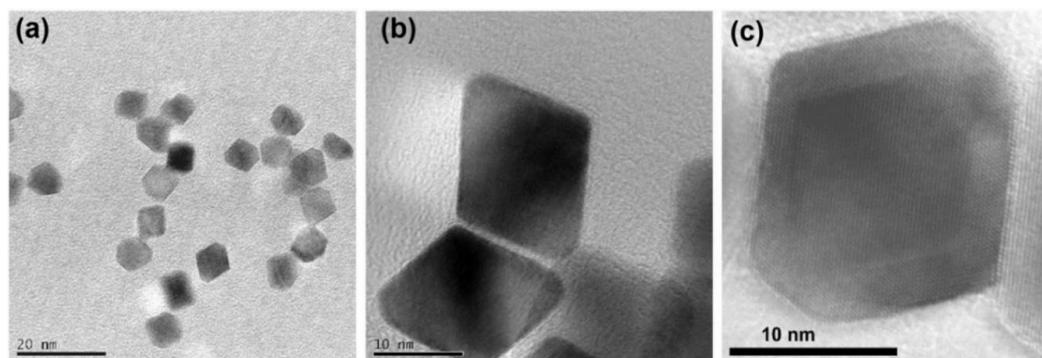
**Figure 5.** (a) Pt nanoparticles by modified polyol method [35], and (b) [42]. (c) Pt-Pd core-shell
