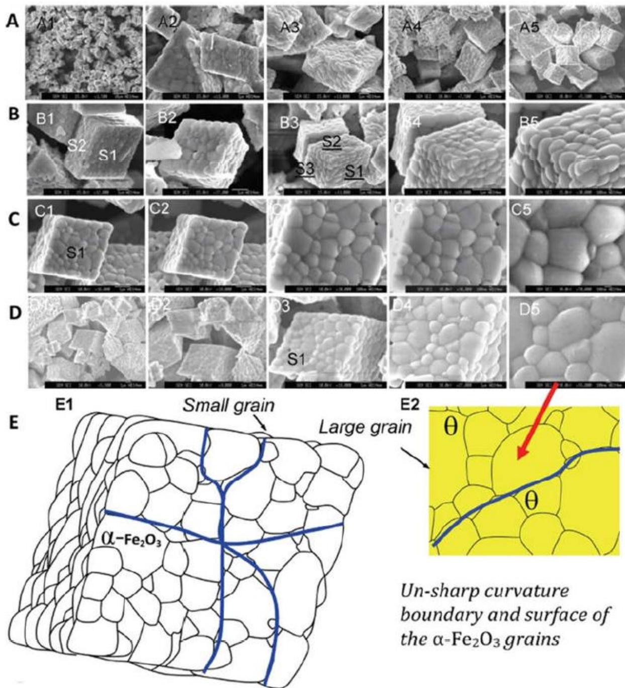
**Figure 7.** The evidences of  $\alpha\text{-Fe}_2\text{O}_3$  oxide micro/nanostructures with grain and grain boundary are a challenge to science [49]. (A–E) The surfaces of  $\alpha\text{-Fe}_2\text{O}_3$  particles with grain and grain boundary.
