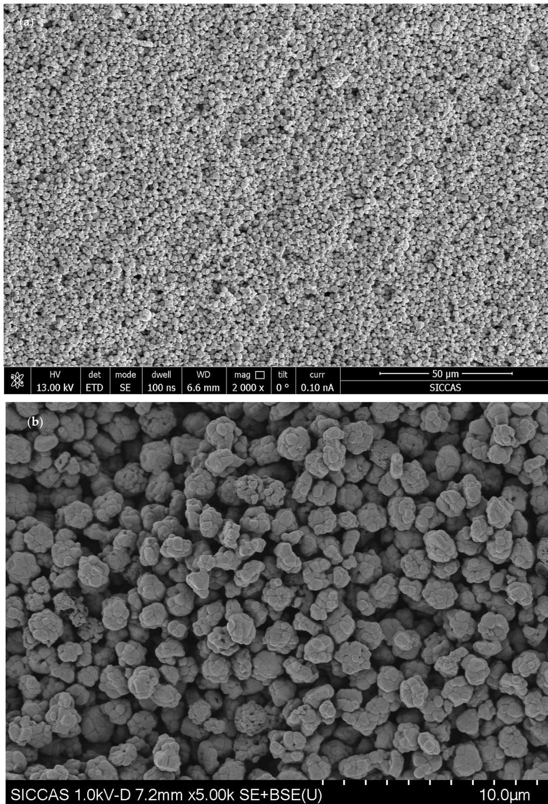
**Figure 9.** (a) The controlled synthesis of  $\text{AB}_2\text{O}_4$ -type  $\text{CoFe}_2\text{O}_4$  micro/nanostructures by modified polyol methods [56]. (b)  $\text{CoFe}_2\text{O}_4$  micro/nanostructures with heat treatment at high temperature in a range of 900–1100 °C (SEM data in our new experimental). It is clear that Pt nanoparticles can be potentially integrated in a ferrite matrix of  $\text{CoFe}_2\text{O}_4$  for electrocatalysis.
