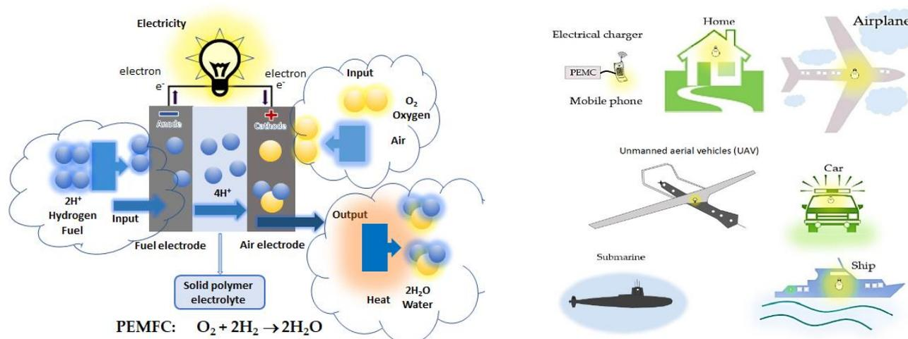
**Figure 1.** Operation of PEMFCs, and promisingly potential applications for electrical charger in mobile phones, FC cars, FC boats, FC ships, FC airplanes, FC homes and offices, and FC plants in integration with electricity from electric power sources, batteries, and capacitors.
