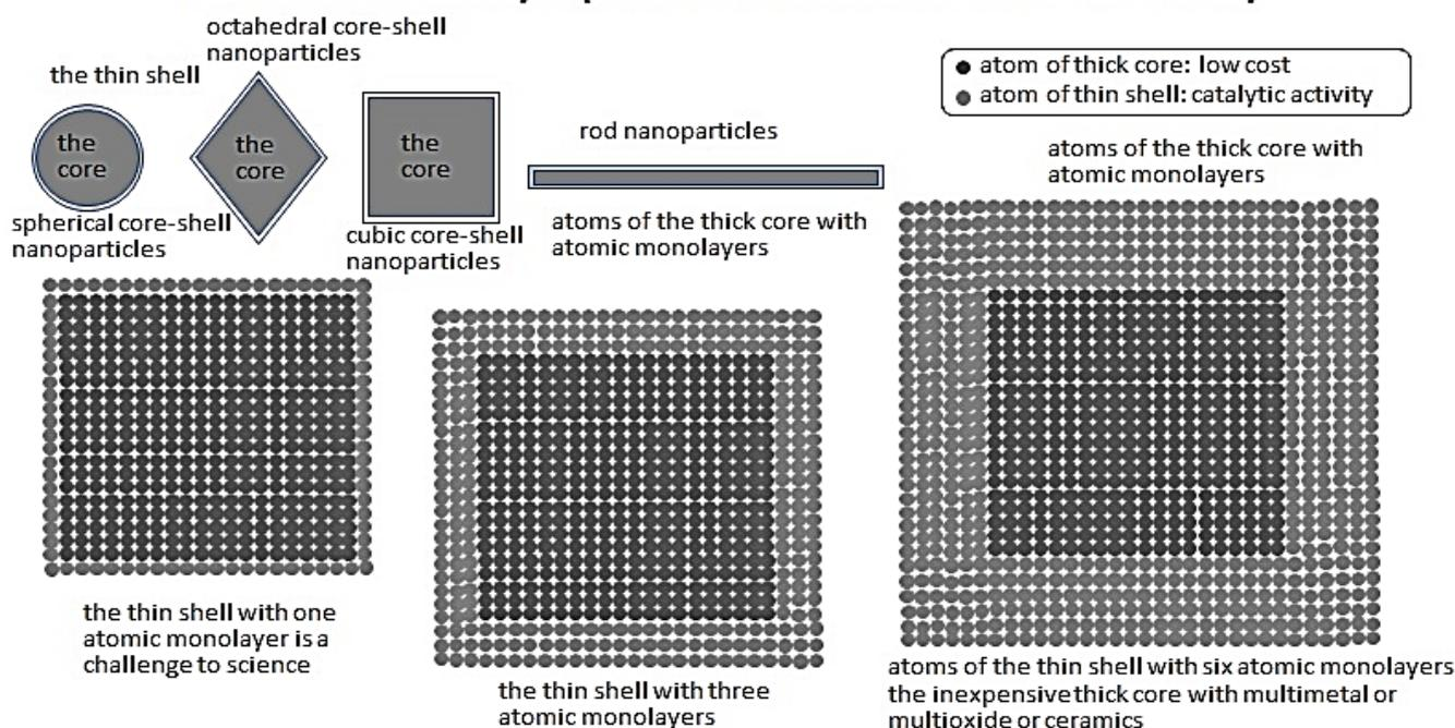
**Figure 10.** The typical models of the cubic Pt-Pd core-shell nanoparticles with the thin Pd shells with several Pd atomic monolayers on the thick cores. This is also a challenge to science. The thin shells of Pt or Pd on the thick metal, bimetal, multimetal, alloy and oxide cores can be realized by modified polyol methods using agents added during the designed process effectively.
