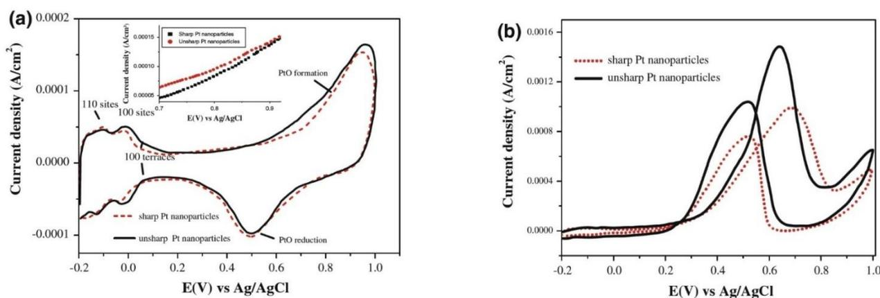
**Figure 2.** (a) Cyclic voltammogram of Pt nanoparticles in electrolyte solution of 0.1 M HClO<sub>4</sub> (scan rate: 50 mV/s, N<sub>2</sub> bubbling time: 30 min). (b) Cyclic voltammogram of Pt nanoparticles the solution of 0.1 M HClO<sub>4</sub> and 1 M CH<sub>3</sub>OH (scan rate: 50 mV/s, N<sub>2</sub> bubbling for 30 min prior to catalytic measurement [33]).
