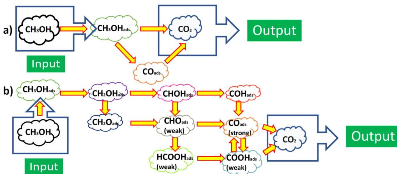
**Scheme 1.** Oxidation of methanol in to  $\text{CO}_2$ . (a) Simple mechanism. (b) Proposed mechanism.
