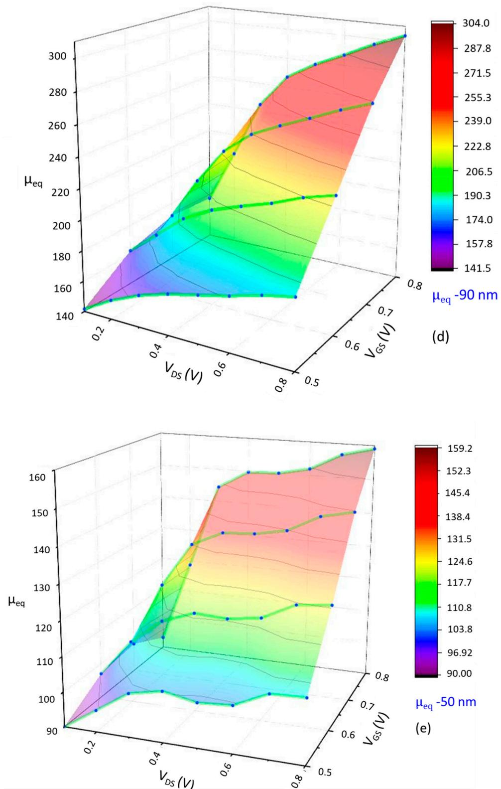
**Figure 8.** Three dimensions of  $\mu_{eq}$  versus  $V_{DS}$  and  $V_{GS}$  at: (a)  $L_{mask} = 500 \text{ nm}$  (long-channel) and  $33 \text{ nm}$  (short-channel), (b)  $L_{mask} = 1 \mu\text{m}$ , (c)  $L_{mask} = 120 \text{ nm}$ , (d)  $L_{mask} = 90 \text{ nm}$ , and (e)  $L_{mask} = 50 \text{ nm}$ .
