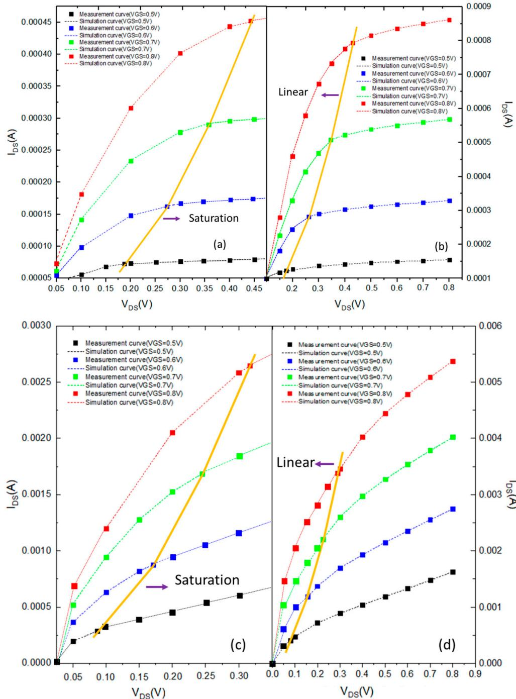
**Figure 7.**  $I_{DS}$  vs.  $V_{DS}$  curves for long-channel devices: (a) at  $L_{mask} = 1 \mu\text{m}$  in section  $X = a$ , and (b) at  $L_{mask} = 500 \text{ nm}$  in section  $X = b$ ; for short-channel devices: (c) at  $L_{mask} = 50 \text{ nm}$  in section  $X = c$ , and (d) at  $L_{mask} = 33 \text{ nm}$  in section  $X = d$ . The yellow lines mean the pinch-off boundary at  $V_{Dsat} = V_{GS} - V_T$ , where  $V_T$  is the threshold voltage.
