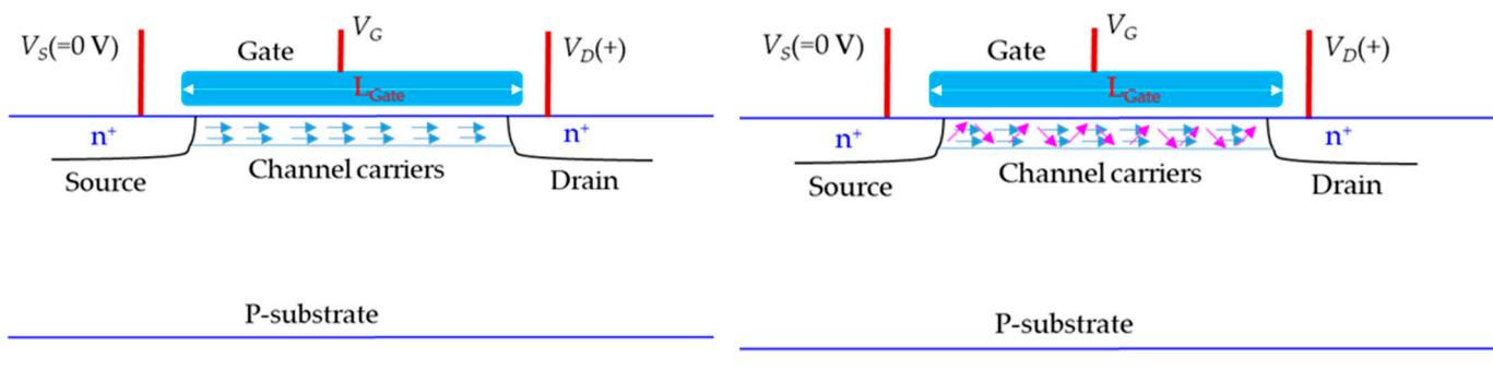
**Figure 1.** Channel carrier conduction due to drift effect in n-channel MOSFET (nMOSFET): (a) without gate bias or with smaller gate bias, and (b) with gate bias as a variable for long-channel device.
