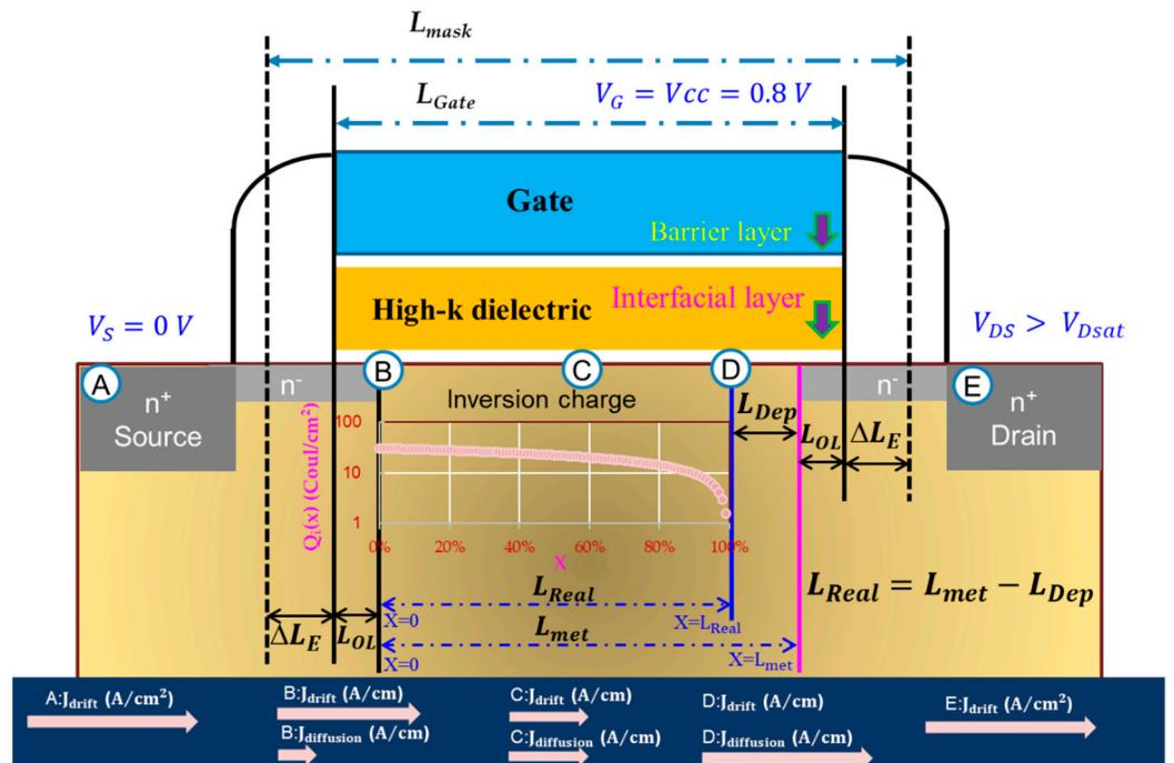
**Figure 3.** Distribution of inversion charge from checking points B to D.
