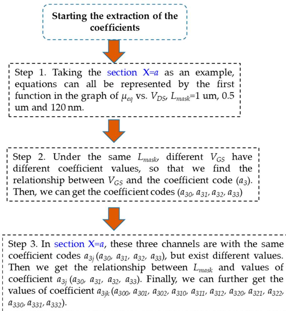
**Figure 5.** Flow chart for extracting the coefficients of  $X_i$  and  $X_{ij}$ , in section  $X = a$ .
