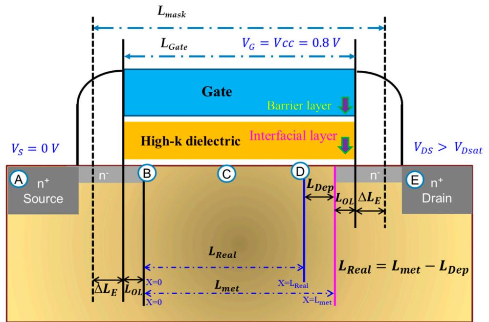
**Figure 2.** Schematic cross-section diagram of an nMOSFET with the definition of channel lengths.
