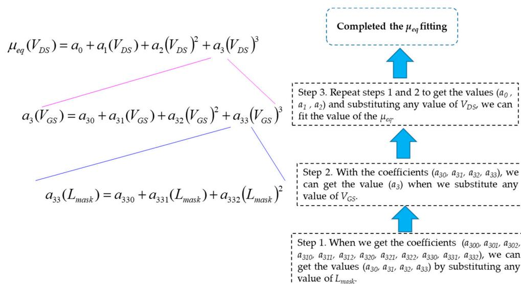
**Figure 6.** Fitting the coefficients of  $\mu_{eq}$  in section  $X = a$  as an example. On the left-hand side, the expansion relationship between  $a_3$  and  $a_{33}$  is illustrated.
