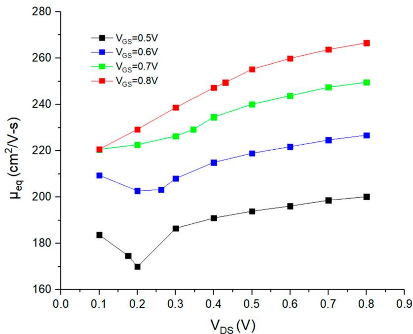
**Figure 4.**  $\mu_{eq}$  vs.  $V_{DS}$  characteristics under different  $V_{GS}$  at  $L_{mask} = 500$  nm in section  $X = a$ .
